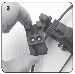
Insert the two nuts into the two holes in the limb base plate (Pic 3). Then turn the base plate over and fit into the front stock using the slots as shown.
