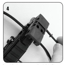
Insert the two screws, and nuts into the limb base plate and tighten down using the allen/hex key supplied (Pic 4/5).
