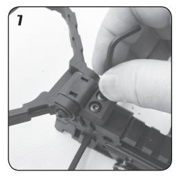
Using the two screws supplied with the foot stirrup, tighten down using the allen/hex key supplied (Pic 7).
