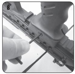
Place the tactical foregrip on the rail and tighten down using the allen/hex key supplied (Pic 8).
