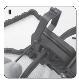
The front sight fits into the two slots on the stock and tighten down using the screws supplied (Pic 9).
